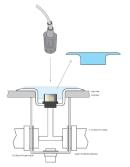
A military connector with gold-plated connections is mounted in the pool deck. One short cable runs from this deck plate to the connection hub (DP-4.5QC) under the starting block. This system provides greater convenience and less possibility of corrosion from pool chemicals and water. The connector is covered when not in use to prevent corrosive build-up.
